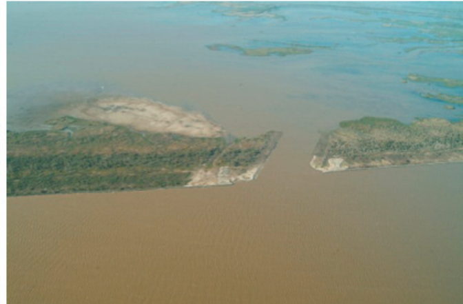
The conveyance channel allows fresh water and sediment to flow from the Mississippi River (bottom of picture) to restore vegetated wetlands in an area that is currently shallow open water.
